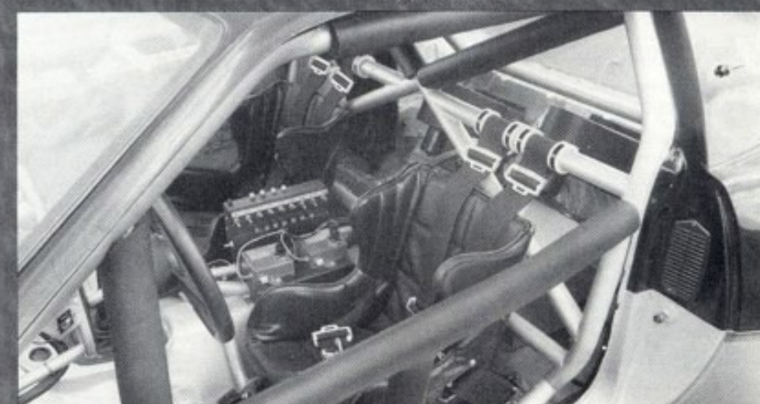
The full rollcage was constructed to IMSA specifications and designed to tie the structure of the car together with hard points corresponding to all suspension attachment points. Padded fiberglass racing seats are used with harnesses.
