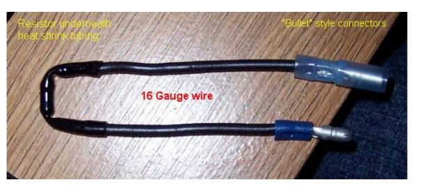
Notice in the above "resistor pack" I lucked out and only needed 1 resistor to match the pellet's resistance. You may not be
